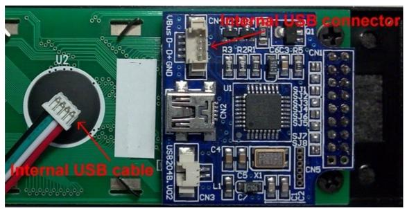
Plug in the internal USB cable to CN4 (Red-VBus/VCC, White-D-, Green-D+, Black-GND)
