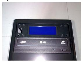
5. Stick the cover sheet on the front end of frame carefully.
