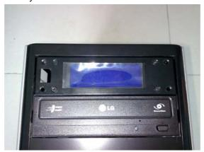
4. Peel off the protective layer of LCD.
