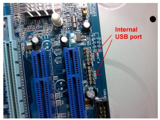
9. Plug the internal USB cable to your board. Please reference the pins configuration of mother board user manual.
