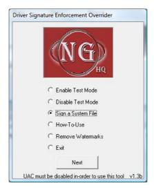
10. You need to sign the driver "libusb0\_x64.sys" in folder of lcd2usbdriver. Insert a driver filename "libusb0\_x64.sys" including full path where it located and click "OK".
