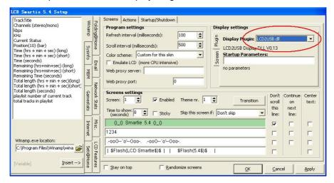
3. Set the screen according to your LCD. LCD contrast and backlight brightness can be tune here.
